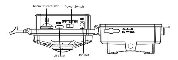
Figure 2 Diagram of camera interfaces
